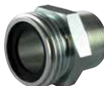
PART: STA2060S Adapter 1 1/4" MPT x 2 1/4" M ACME
