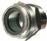
Adapter ..... ME502S-16/10 2" MPT x 2 1/4" M ACME 1 1/4" Female Threads
