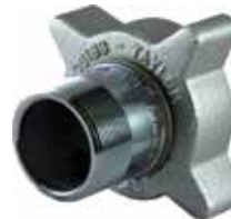
Fill Coupling ..... STA1156FS 2 1/4" F ACME x 1 1/4" MPT
